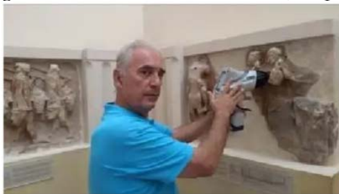
Ioannis Liritzis at work: XRF measurements of an embossed forked metopes of the Sikyonian treasure Delphi Museum
